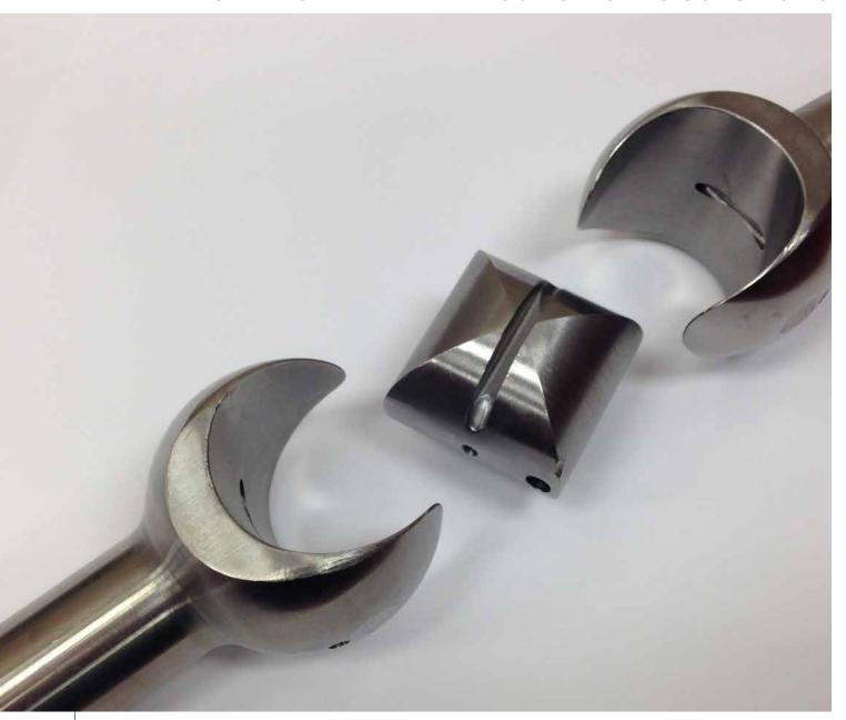
Using SOLIDWORKS 3D design and simulation solutions, CCTY Bearing not only realized substantial reductions in development and delivery lead-times, the company also created its patent-pending Square Ball Universal Joint. The innovative design allows for the smooth transfer of high torque while making assembly easier, by reducing the number of U-joint components from approximately 115 to six.
